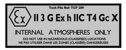
This equipment is designed to meet the requirements of Group II Category 3G in respects to ignition sources internal to the pump. This classification is in accordance with Directive 2014/34/EU.
