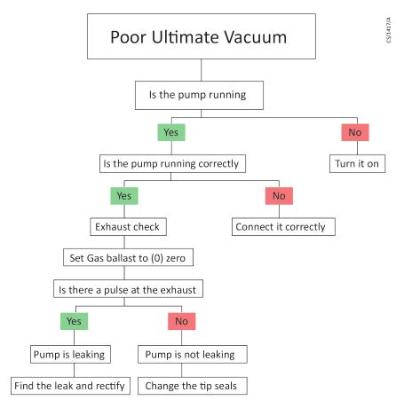
Figure 13 Poor ultimate vacuum flow chart
