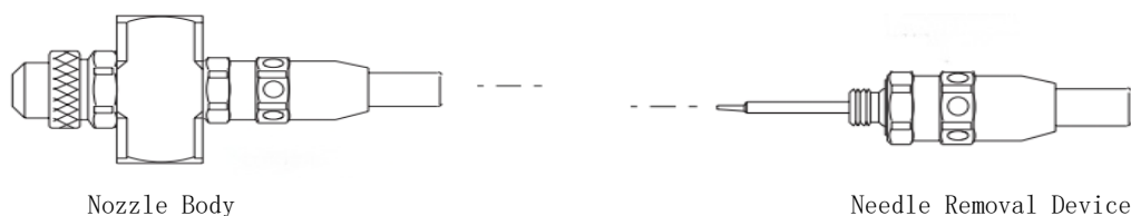
Figure 4-1-3-2.1: Schematic diagram of nozzle body and spray device
