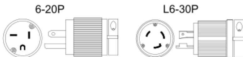
Figure 5 - Plug types used on chillers
