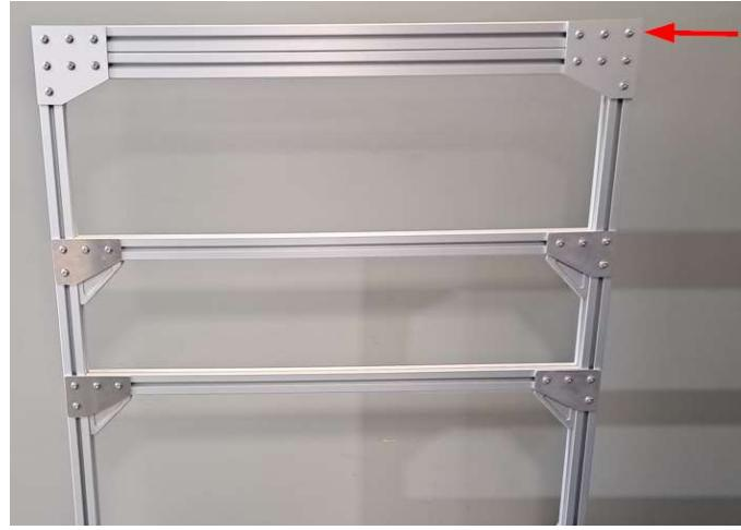
18. **Use a level** to adjust and tighten the 2x, 35¾" bars attached to 4-hole brackets.
