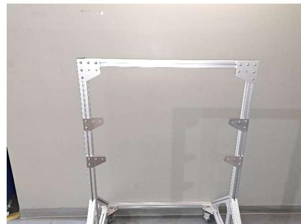
**14. Loosely attach 1x, 35¾" bar just below the top bar between the 7-hole plates:**
