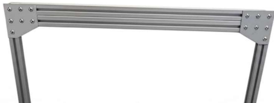
**15. Loosely attach 2nd 35¾" bar to the first set of 4-hole brackets:**
