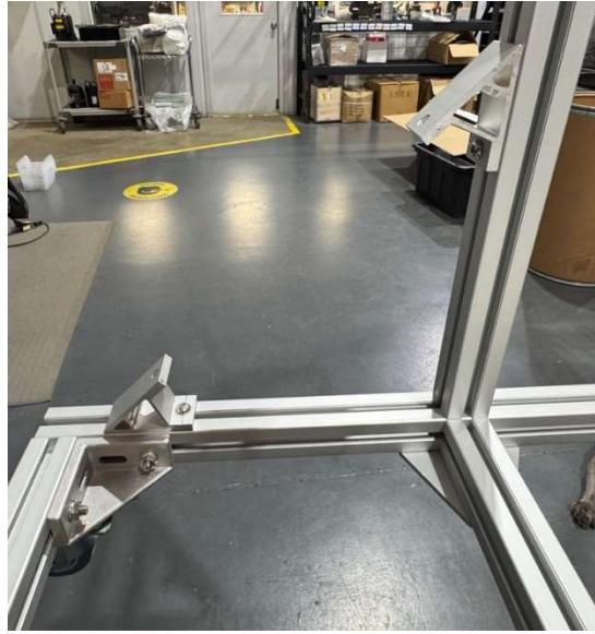
**26. Loosely attach the 4 angle-cut bars to the other side of the 45° brackets:**
