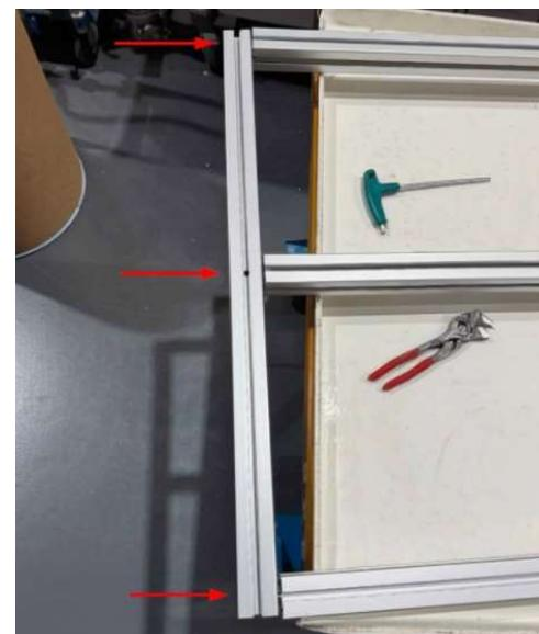
4. **Attach the second 30" 4-hole bar (in the same orientation)** to the other end of the 3 threaded 35¾" bars.
