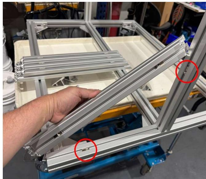
**25. Loosely attach eight 45° brackets using:**
