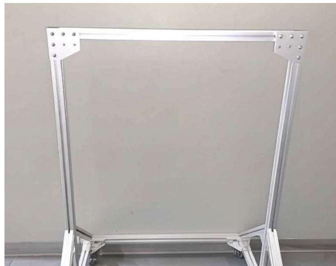
**13. Loosely attach 4x, 4-hole brackets to the 50" upright bars at desired height for crossbars.**
