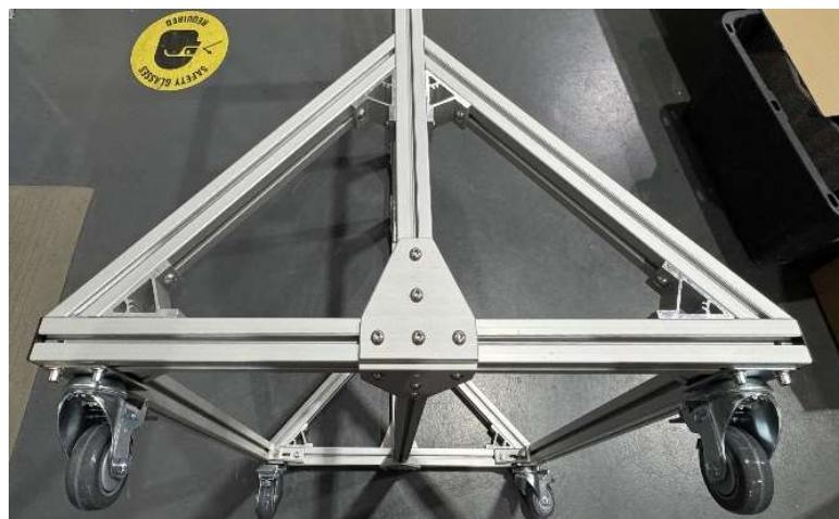
27. **Adjust angle-cut bars** so that their tip ends are **flush and level** with the top edge of the 30" 4-hole bottom bar.
